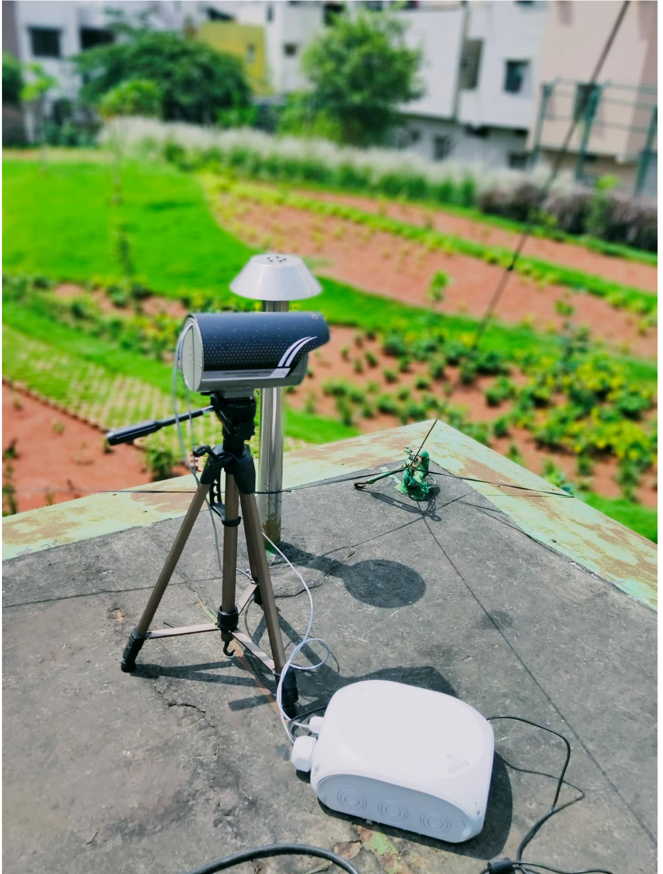
The indigenously developed Photonic System, AUM collocated with the CAAQMS at SGHALLI
